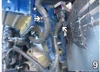
9. After the washer reservoir is removed, unclamp the two hoses and pull up out of way. Do this on both sides.
