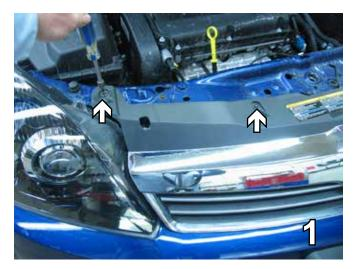
1. Using a 25 Torx, remove three metric bolts from the top side of the fascia. Set the bolts aside to be reinstalled later.
