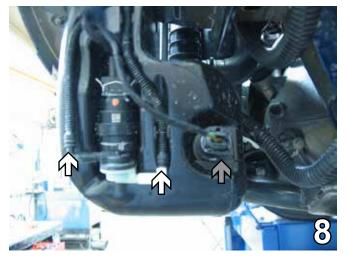
Pull the three washer reservoir hoses out. Disconnect two (white arrows) and plug their ends. Unplug the electrical connection (gray arrow). Set the washer reservoir aside to be reinstalled later.
